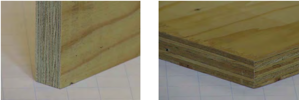
Fig. 6.8 LVL and LVL with layers in transversal direction
