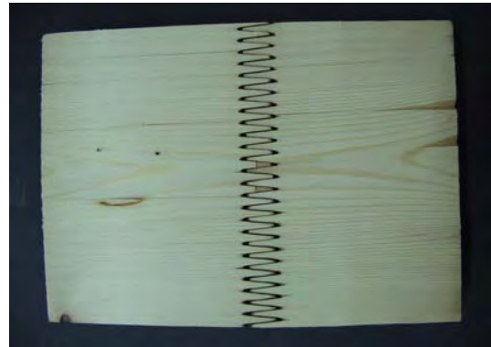
Fig. 4.3 Scarf-joint at the outermost layer of LVL and finger-joint at the section of a glulam lamella
