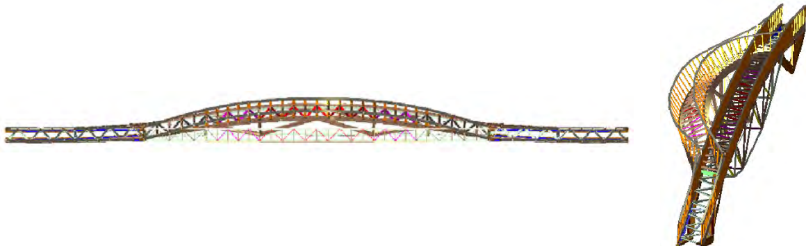
Fig. 15.16 First horizontal mode shape of Lardal bridge – eigenfrequency 0,83 Hz (the lowest eigenmode)
