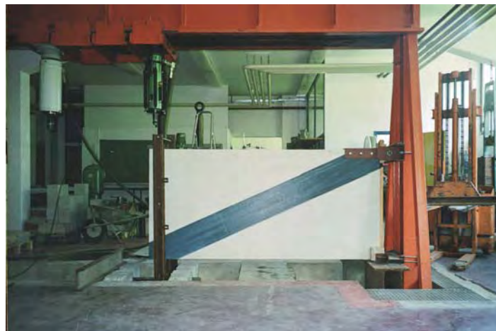
Fig. 13.11 Experimental test on diagonally CFRP reinforced test sample [17], rotation for 90°
