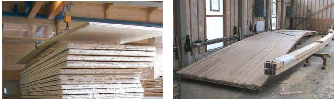
Fig. 6.16 Planar and curved CLT-elements in the production process
