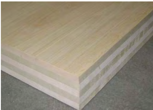
Fig. 4.4 Cross-wise joints for CLT, batten- and laminboards
