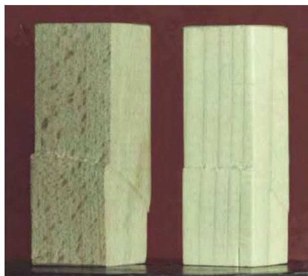
Fig. 9.3 Failure mechanism of timber member in compression
