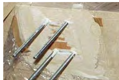
Glued-in rods (loaded transversal to their axis)
