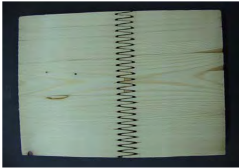
Fig. 10.5 Finger-joint of a glulam lamella and glued frame corner
