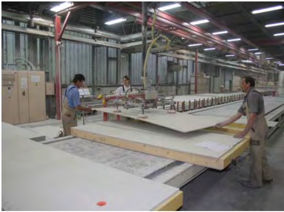
a. Factory manufacturing of pre-fabricated walls
