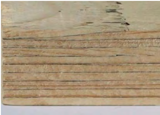
Fig. 4.3 Scarf-joint at the outermost layer of LVL and finger-joint at the section of a glulam lamella
