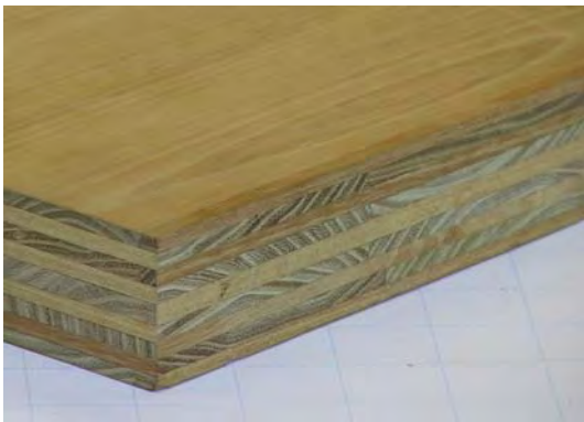
Fig. 6.6 9-layered plywood (robinia) and the use of plywood as stiffening elements in a shear-wall
