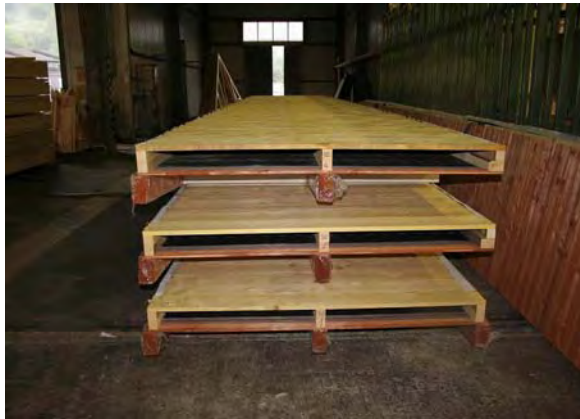
a. Prefabricated roof beams with boards
