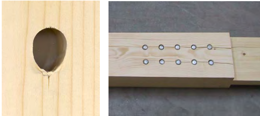
Fig. 10.10 Splitting of a test specimen in the embedment zone of a fastener and “zip-effect” in a tested joint
