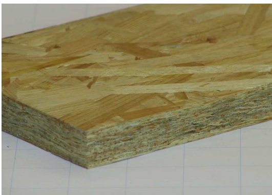
Fig. 3 OSB and its utilisation as load-carrying sheathing material in a shear -wall
