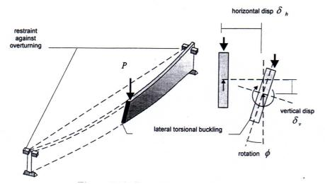
Figure 6.11 Lateral-torsional buckling of simply supported beam
