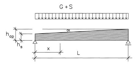
Fig. 10.1 Scheme of the single tapered beam
