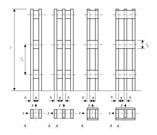
Figure 11.1 – Spaced columns
