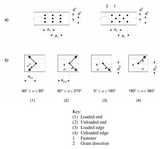
Figure 8.7 – Spacings and end and edge distances
