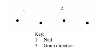
Figure 8.6 Nails in a row parallel to grain staggered perpendicular to grain by d
