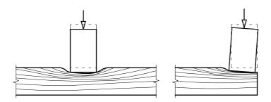
Figure 6.3 Bearing effects at supports and points of concentrated load application
