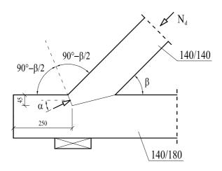
Design compressive strength at an angle to the grain
