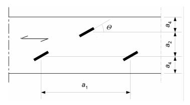
Figure 8.10 Definition of spacing for staples
