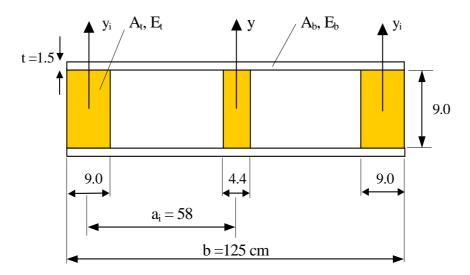
Figure 2: Cross-section of the single wall element.
