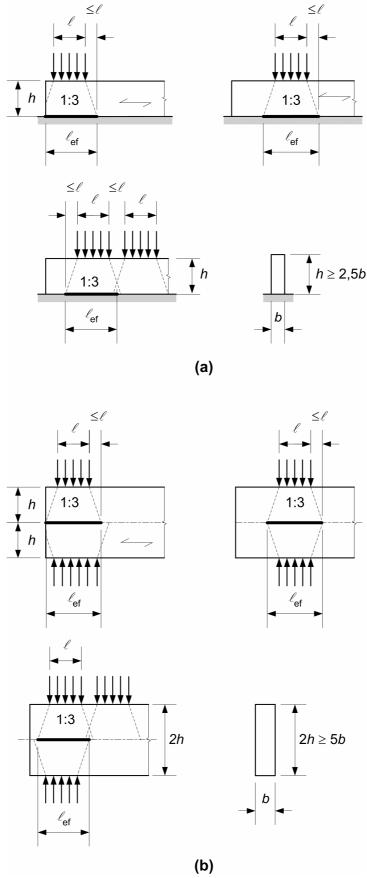
Figure 6.6 Determination of effective lengths for a member with h/b > 2,5 on (a) a continuous support, (b) discrete supports
