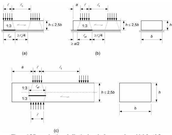
Figure 6.5 Determination of effective lengths for a member with  $h/b \le 2,5$ , (a) and (b) continuous support, (c) discrete supports
