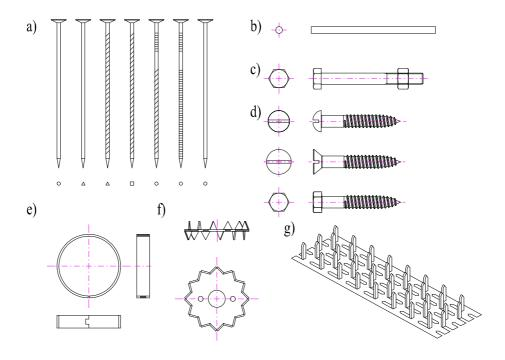
Figure 8.1 Metal fasteners
