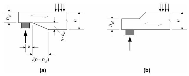
Figure 6.15 End-notched beams
