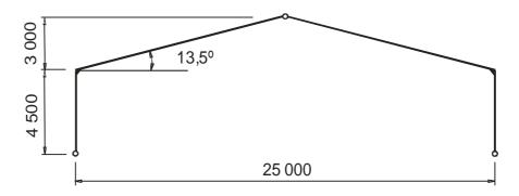
$\begin{array}{lll} \text{Span:} & L=25 \text{ m} \\ \text{Depth of the rafter:} & h_R=1480 \text{ mm} \\ \text{Width of the rafter:} & b_R=200 \text{ mm} \\ \text{Depth of the column:} & h_C=1480 \text{ mm} \\ \text{Width of the column:} & b_C=2\times120 \text{ mm} \end{array}$
