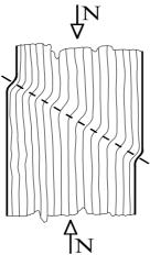
Figure 6.2 Failure mechanisms in compression
