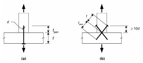
Figure 8.8 (a) Nailing perpendicular to grain and (b) slant nailing
