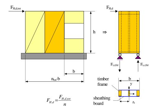
Figure 1: Example of the wall assembly.
