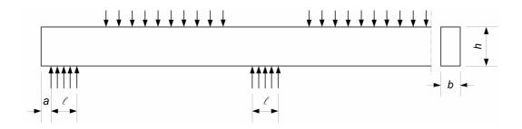
Figure 6.4 Beam on supports
