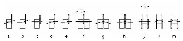
Figure 8.3 Failure modes for steel-to-timber connections
