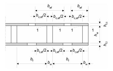
Figure 9.2 Thin-flanged beam
