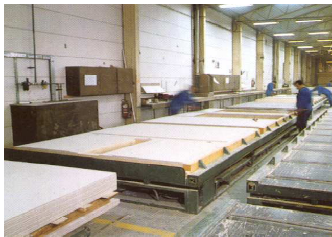
Fig. 11: Construction of the wall elements in the assembly-plant.
