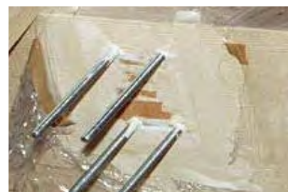
Glued-in rods (loaded transversal to their axis)
