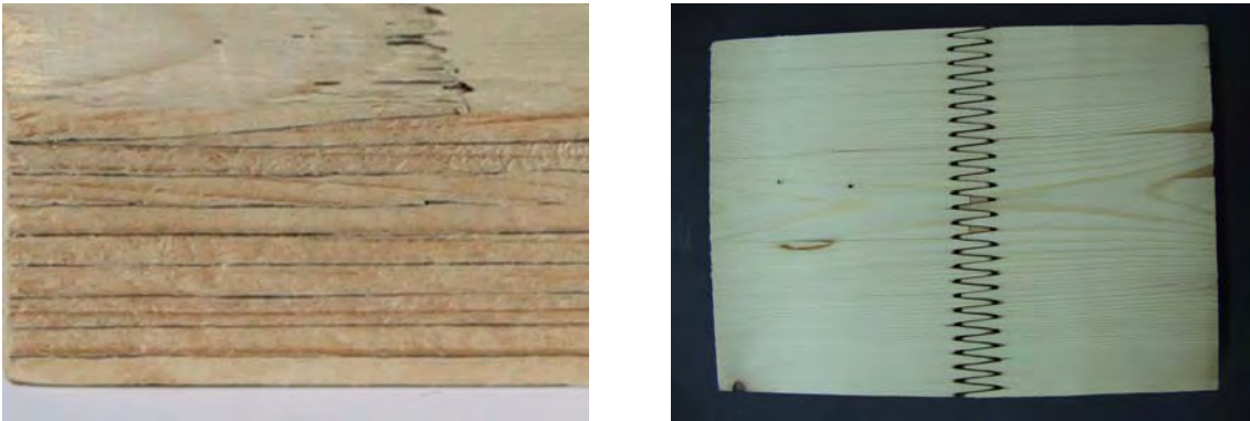
Fig. 3 Scarf-joint at the outermost layer of LVL and finger-joint at the section of a glulam lamella
