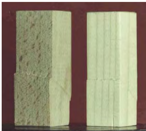
Fig. 3 Failure mechanism of timber member in compression
