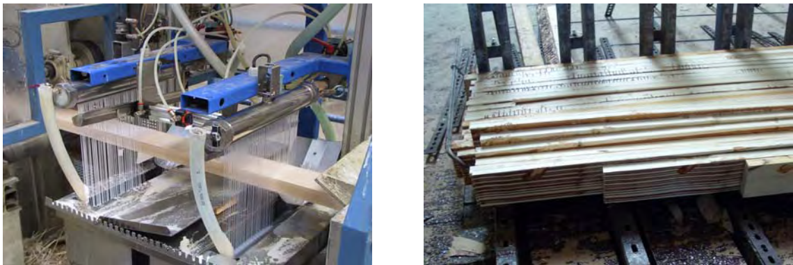
Fig. 2 Application of adhesive and pressing of glulam
