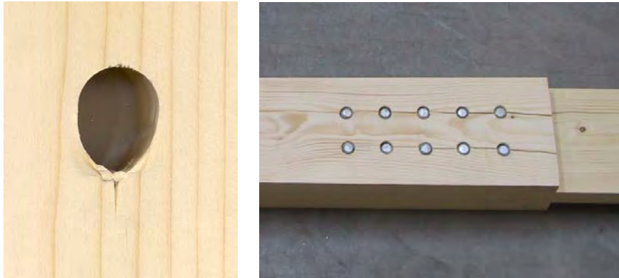
Fig. 10 Splitting of a test specimen in the embedment zone of a fastener and “zip-effect“ in a tested joint
