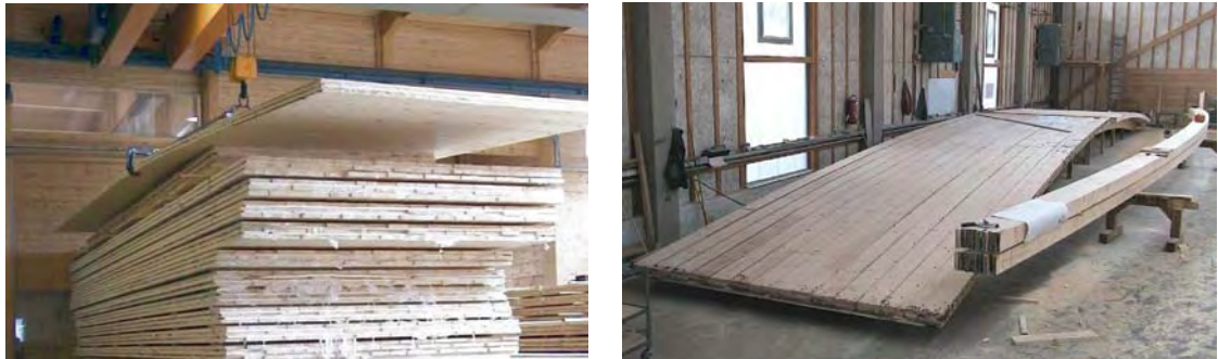
Fig. 17 Planar and curved CLT-elements in the production process
