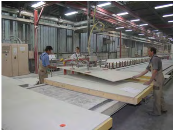
a. Factory manufacturing of pre-fabricated walls
