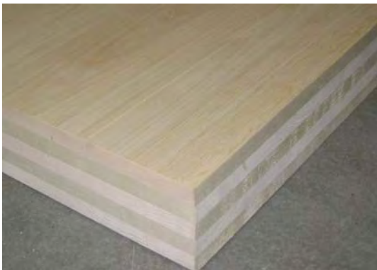
Fig. 4 Cross-wise joints for CLT, batten- and laminboards
