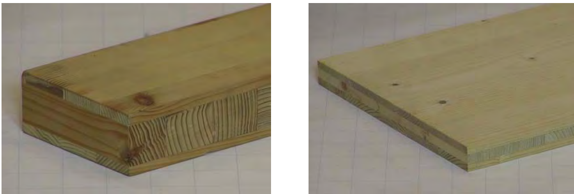
Fig. 7 Battenboard and laminboard
