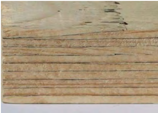
Fig. 3 Scarf-joint at the outermost layer of LVL and finger-joint at the section of a glulam lamella
