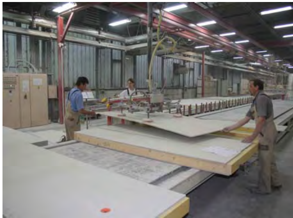
a. Factory manufacturing of pre-fabricated walls
