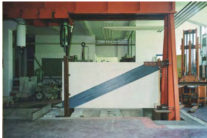
Fig. 11 Experimental test on diagonally CFRP reinforced test sample [17], rotation for 90°
