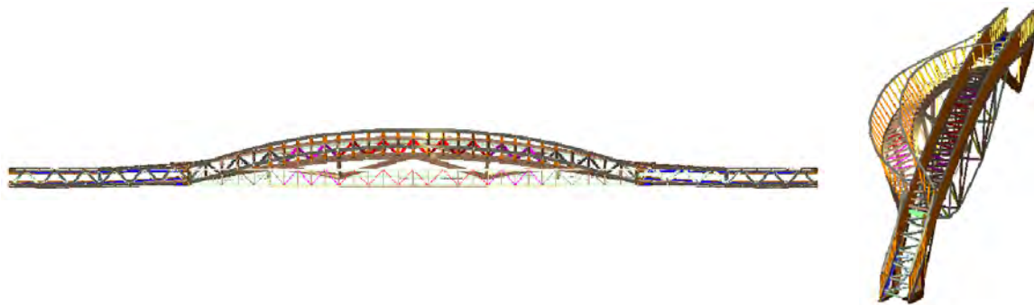
Fig. 16 First horizontal mode shape of Lardal bridge – eigenfrequency 0,83 Hz (the lowest eigenmode)
