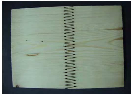
Fig. 3 Scarf-joint at the outermost layer of LVL and finger-joint at the section of a glulam lamella
