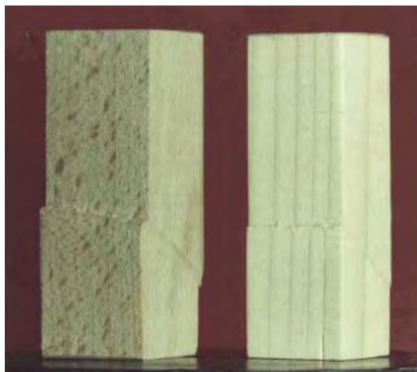
Fig. 3 Failure mechanism of timber member in compression
