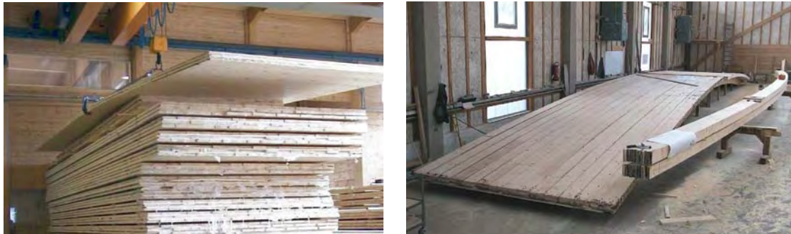
Fig. 16 Planar and curved CLT-elements in the production process
