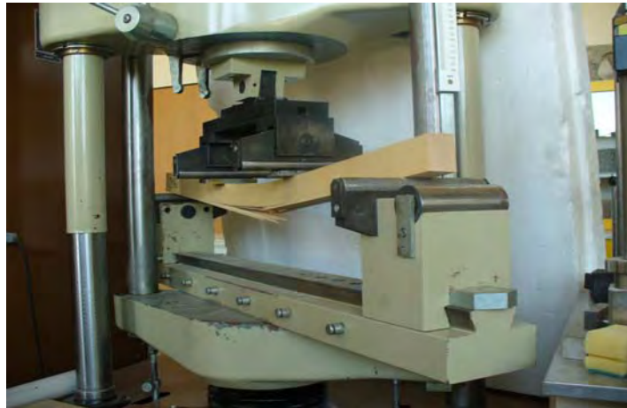
Fig. 5 Solid timber bending test
