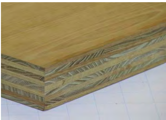
Fig. 6 9-layered plywood (robinia) and the use of plywood as stiffening elements in a shear-wall
